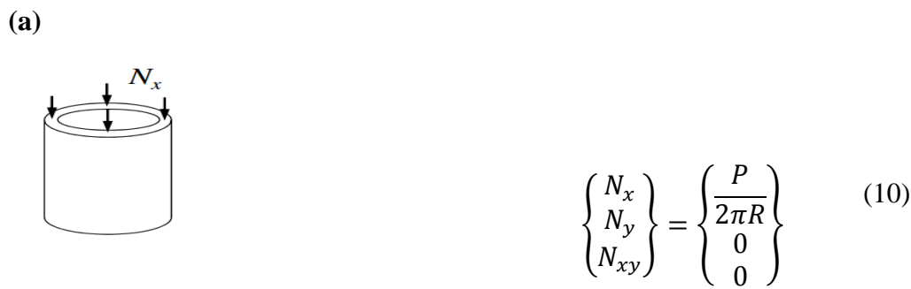
(b) Figure 4. Generalised stresses under internal pressure (a) and axial compression (b)
